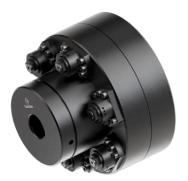
A robust torque limiter with modular torque adjustment. Free rotation after overload permits high rotational speeds with also high torque settings and large shaft diameters can be accommodated. The torque modules can be individually adjusted and re-engagement of the unit is quick and easy.
