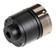
A friction clutch or roller with torque adjustment even during operation. Ability to disengage the drive and driven by pneumatic or electrical impulse. Low residual torque after disengagement. Calibration adjustable by changing the pressure (pneumatic) air supply. Transmission through rollers with re-engagement in phase 360° (equidistant on request, 30°, 45°, ...). Free rotation for long periods after overload.
