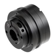
Safety coupling with the transmission of motion through rollers that allow complete disengagement when the calibrated torque is reached permitting a quick stop of the transmission due to micro-EM1. Suitable for transmitting high torque with high reliability and compact size.
