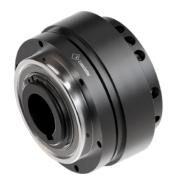
A backlash free safety coupling with free rotation and low residual torque suitable for high speed transmission. The disengagement is instantaneous once the torque is reached, the calibration is adjusted by changing the pressure of the springs. The reengagement is manual, quick and reliable.
